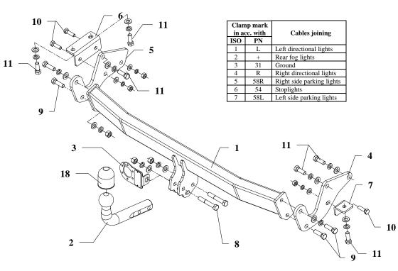
This towing hitch is designed to assembly in following cars: **TOYOTA PICNIC, 5 doors, VAN (XM1),** produced since 10.1996 till 05.2001, catalogue no. **O54** and is prepared to tow trailers max total weight **1500 kg** and max vertical mass **60 kg**.
